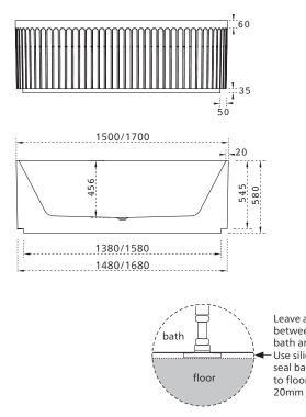
Leave a 3mm gap between base of bath and floor. Use silicone to seal base of bath to floor, leaving a 20mm weephole.
