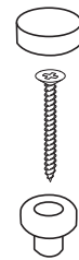
2 x caps (chrome plated) 2 x screws 2 x pan plugs (white) Optional fixing #2 — used to secure pan to concealed fixing bracket. Plastic plug is placed into hole in side of pan exterior, screw is rebated into plug and then screws into a hole in upright section of bracket. Chrome cap is used to cover plastic plug.
