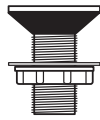
2 x plugs Plugs can be used to plug holes in sides of pan if required.
