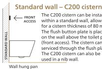
The C200 cistern can be installed within a standard wall, allowing for a cistern thickness of 80 mm. The flush button plate is placed on the wall above the toilet pan (front access). The cistern can be serviced through the flush plate. The C200 cistern can also be used in a nib wall.
