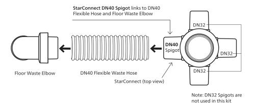
**WARNING** Only the DN40 Spigot is used in this Kit. The three DN32 spigots are only needed with external overflow kits and should be left intact and unchanged. Do not knock out the DN32 spigot ends unless installing an overflow kit.
