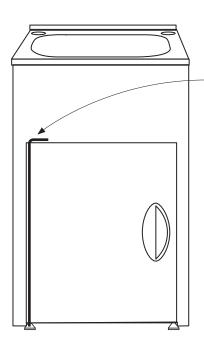
The door is held in place by a **long metal pin** with a bend at the top.
