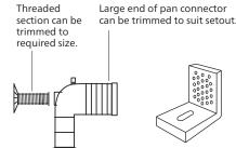
1 x pan connector For connecting pan to floor outlet pipe/S-trap.
