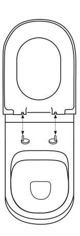
To fit seat, slide seat down onto stainless steel pins.
