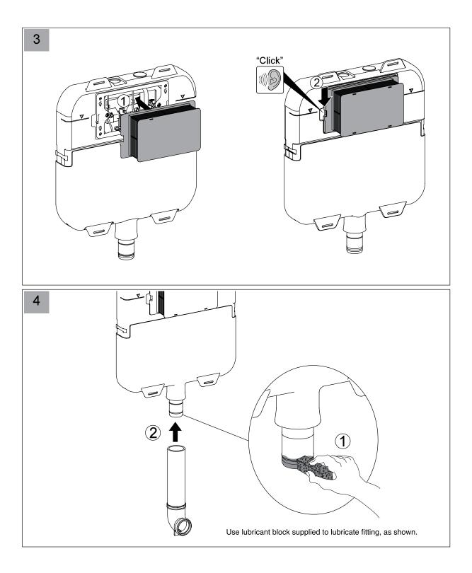
Note: Ensure that the flush pipe is fixed securely to a nogging in the wall in order to avoid it dislodging from the cistern when the pan is fitted.
