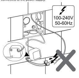
The size of cable should be 1.0-2.5 mm  $^{\!2}$  and the wire connector should be connected firmly.
